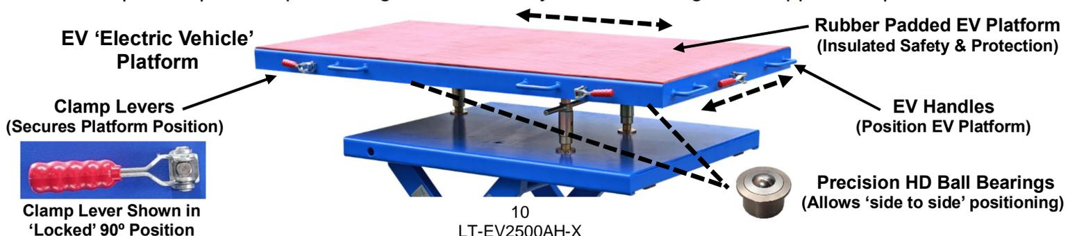
**B. Adjustable EV Platform 'Tilt Angle'** - the 2+adjustable Jack Screws can be rotated so that the upper EV Platform can be slightly tilted lengthwise by 4° and widthwise by 8° providing flexibility to better configure component to vehicle.
