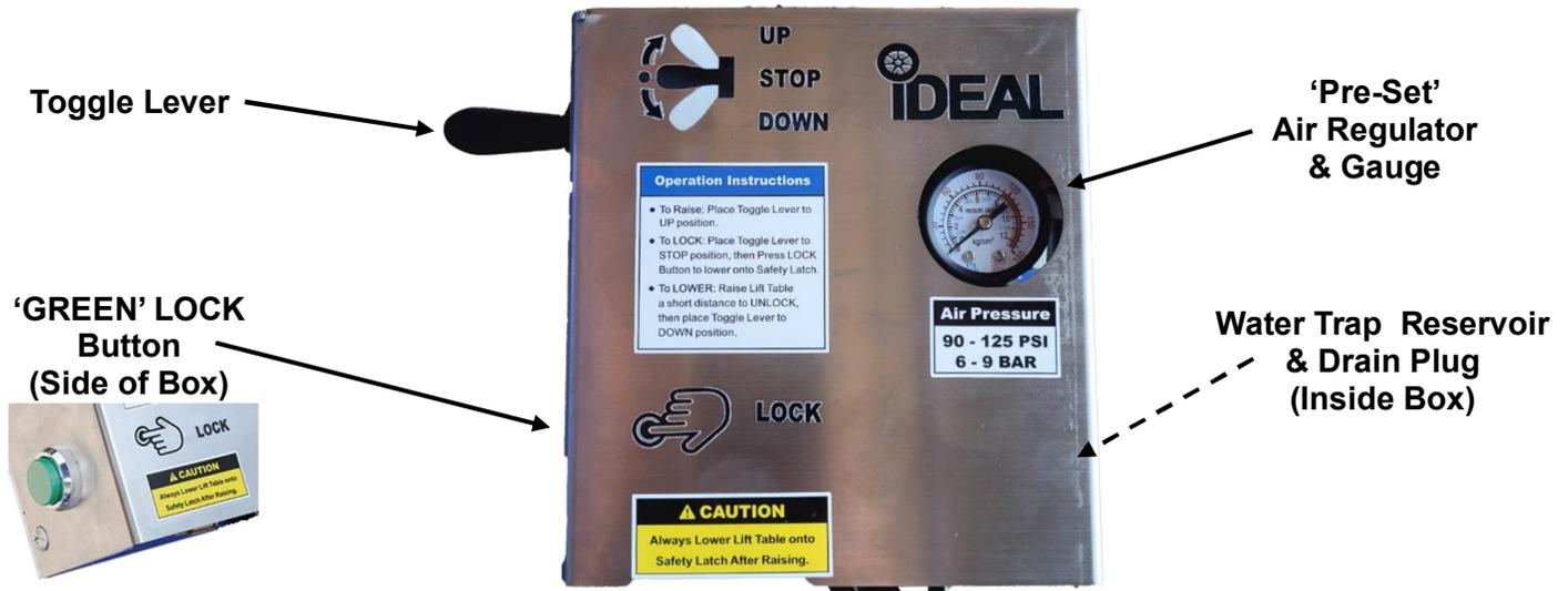
**IMPORTANT:** Ensure compressed air supply is set at 90 to 125 PSI for proper lift table operation and performance. Check air fitting connections for proper tightness.
